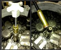
4.) Place smaller input seal over shaft with lip facing down.
