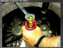
3.) Install handle and turn clockwise until the seal is removed.
