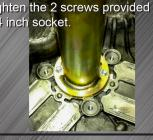
7.) Once screws are installed turn the knob in by hand untill seal is
